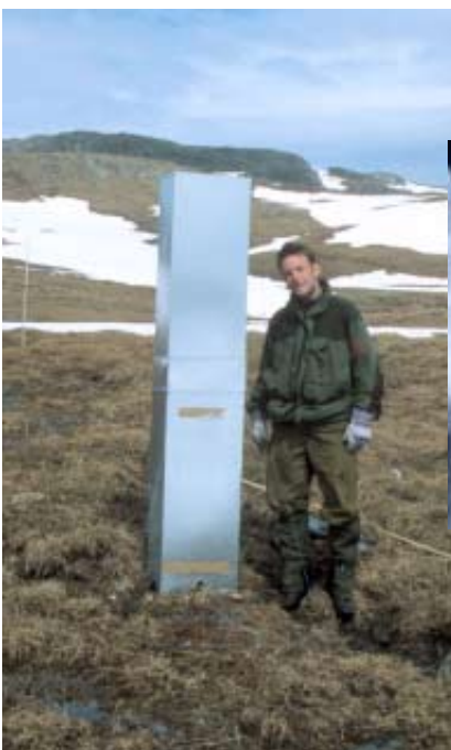
The height of the modular chimney can be altered as snow level changes.
