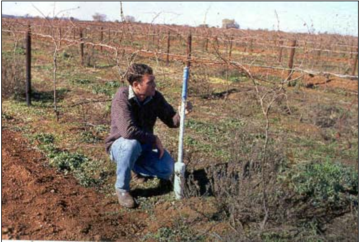
Figure 4. Testwell in vineyard with capacitance logger
